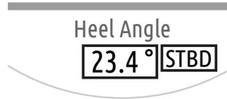
Figure 7: Heel Angle Warning Display
