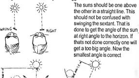
Only use the reflections in the clear glass surfaces. The glue at the upper and lower edges of the sextant bends light like a prism and will not give a true reflection.
