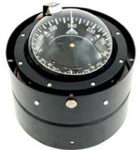
Spherical Magnetic Steering Compass
