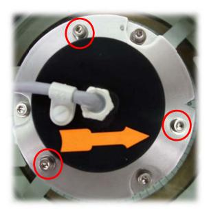
Remove the three marked screws.
