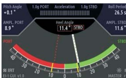
Monitor display with current heel angle (graphic and numeric), current pitch angle, max. port and starboard heel as well as horizontal acceleration
