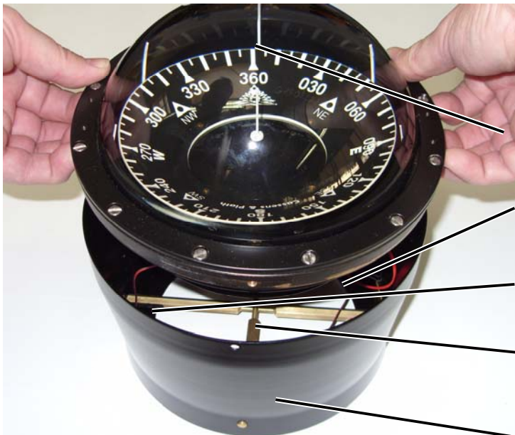
Separate set-up type compass from binnacle with inside flange
