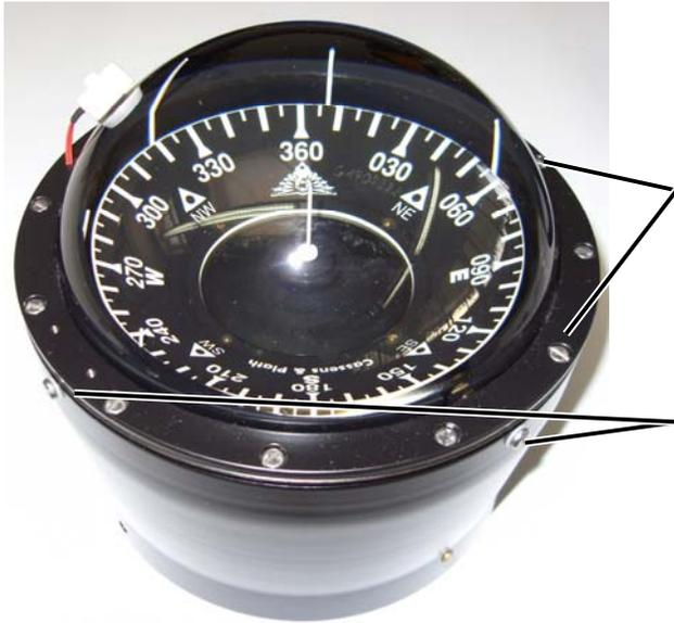
**Separate set-up type compass from binnacle with inside flange**
