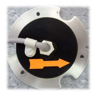
Detector can be removed from distance cylinder.
