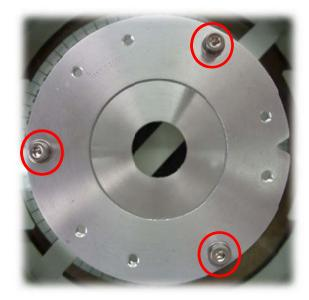
Remove the three marked screws.
