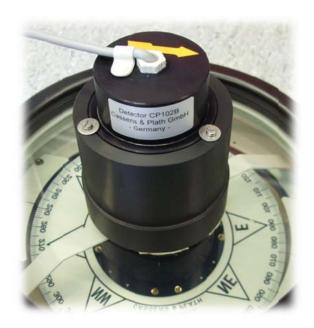
The old version will be replaced by new version during service of magnetic compass.
